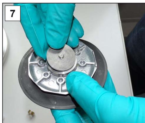
7. Place all spacer discs on the thread pin.
