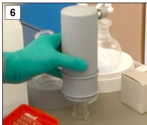
6. Set the chiller down securely so that no liquid can escape.
