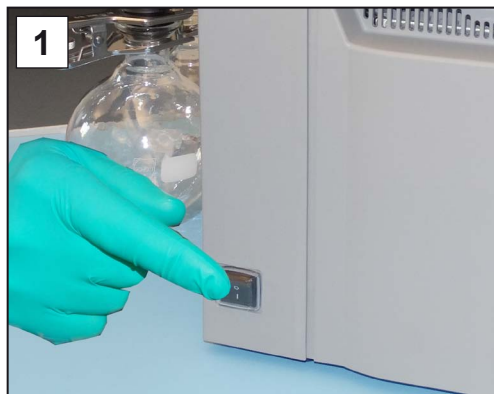
1. Switch the Pumping unit off and unplug the power plug.
