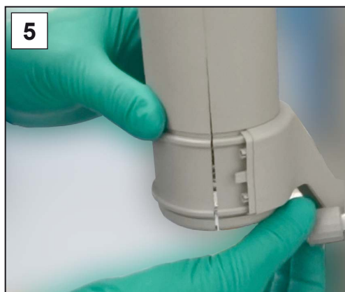
5. Unscrew the knurled nuts, pull off the molded hose, and remove the cooler.
