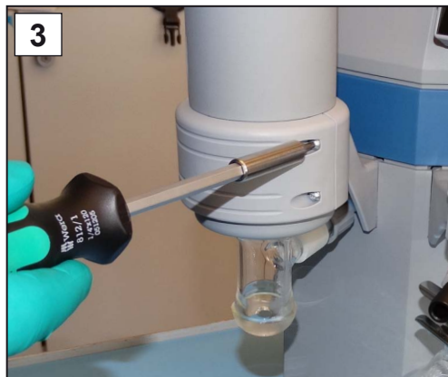
3. Unscrew the screws from the counterholder; Torx screwdriver TX10
