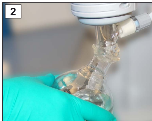
2. Remove the glass flask from the EK as well as the connected hoses.
