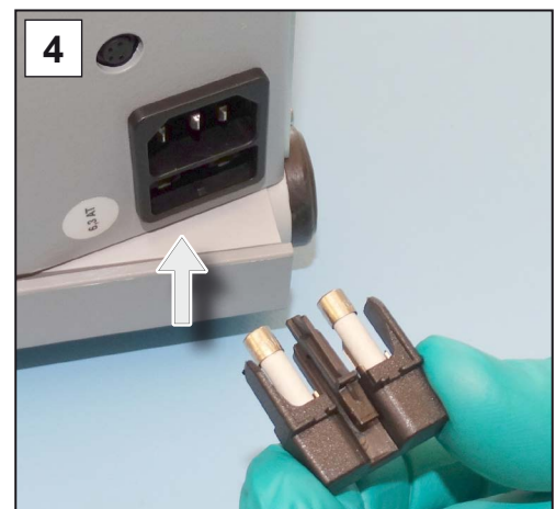
4. Push the fuse holder back onto the fuse socket.
