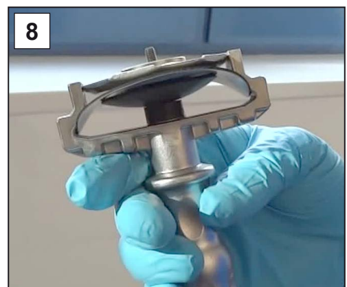
8. Fix the diaphragm assembly inside the diaphragm wrench.
