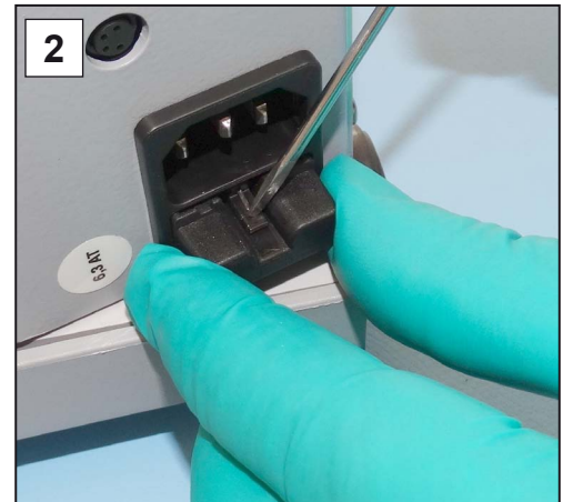
2. Carefully pull out the fuse holder.
