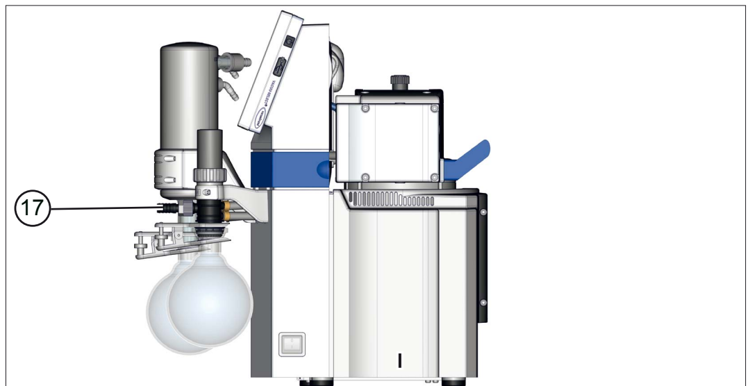
17 Inlet – vacuum connection (distribution head), with electronically controlled valve
